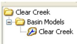
2. Expand Basin Models in the watershed explorer and click on Clear Creek this will open the basin schematic window.
