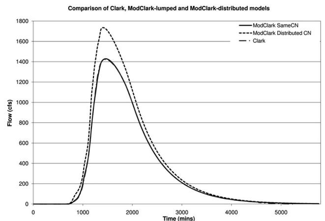
**Fig. 6.** Comparison between Clark and ModClark hydrographs for American Fork River Watershed with both averaged and distributed CN used for all grid cells
