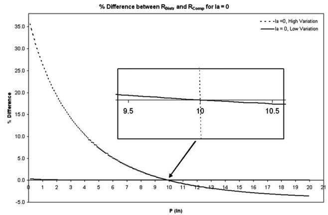
**Fig. 12.** Percent difference between  $R_{Distr}$  and  $R_{comp}$  with low variation in CN over the watershed (unit: 1 in.=2.54 mm)
