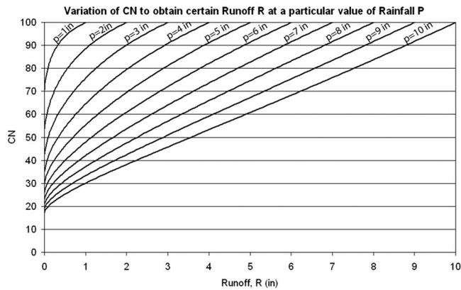
**Fig. 8.** Variation in CN value to obtain a runoff for different values of rainfall (unit: 1 in.=2.54 mm)
