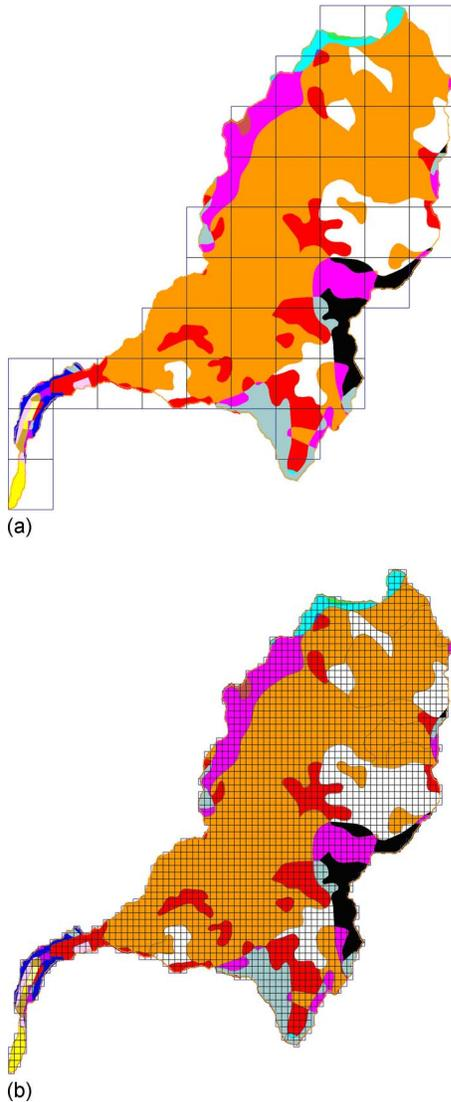
**Fig. 10.** (a) Conventional HRAP grid used in ModClark; (b) new fine resolution grid implemented in WMS
