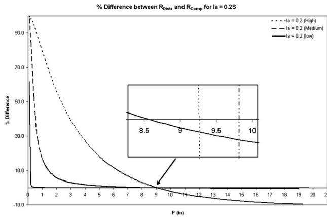
**Fig. 11.** Percent difference between  $R_{Distr}$  and  $R_{comp}$  with high variation in CN over the watershed (unit: 1 in.=2.54 mm)
