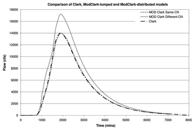
**Fig. 7.** Comparison between Clark and ModClark hydrographs for Virgin River Watershed with both averaged and distributed CN used for all grid cells
