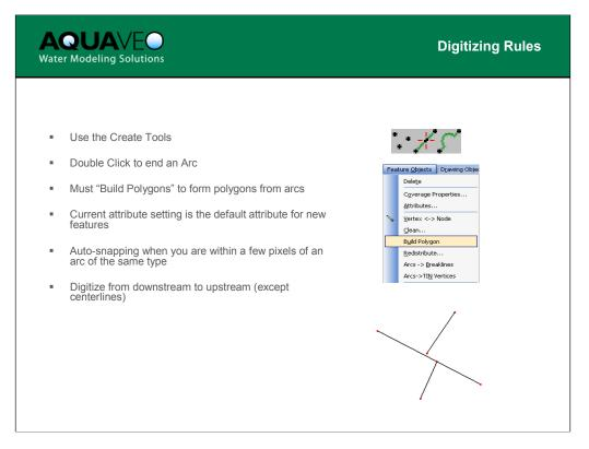
Feature objects are created in WMS using the tools and typical point and click operations in the graphics window. Be sure to use the Create tools (the ones without the arrows). There is no undo command in WMS, however, if you inadvertently create a feature you can select it and delete it.
