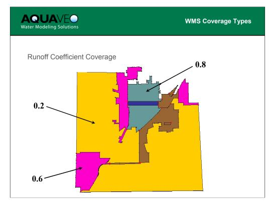
Runoff coefficient coverages are comprised of one or more polygons, each with a runoff coefficient assigned to them. The "weighted" runoff coefficient can be automatically computed for each basin in the model.
