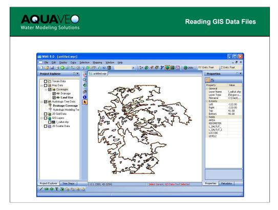
The GIS module can read any type of ESRI-supported GIS data file if ArcObjects is enabled or shapefiles if not. As with the direct reading of shapefiles, a new coverage of the appropriate type should be created in the Map module before converting features from the GIS layer. You can then select only those features you wish to convert to feature objects. As part of the conversion process you will have the opportunity to map attributes from the GIS table to the WMS attributes.
