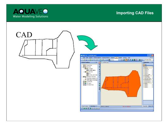
DXF, DWG, and DGN CAD files can be opened and displayed as background maps just like the GIS layer files. However, unlike the GIS layers, it is not possible to perform coordinate conversions on CAD files. CAD files may also be converted to feature objects in the active coverage.
