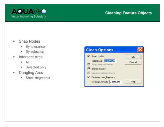
When importing features from CAD or other GIS layers, there are often topologic problems such as nodes that should be coincident but are not. You may also have lines that overlap but do not intersect at a common node. In order for WMS to use the features as part of a coverage, they need to be topologically correct. Some of these corrections will need to be made manually, but the Clean options can be very useful for eliminating the topologic errors.
