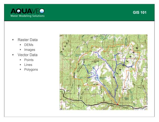
There are two primary data types in GIS: raster and vector data. Raster data includes gridded data sets like DEM elevations as well as images. Raster data are easy to work with and intuitive from a visual perspective, but they are not an "intelligent" data structure.
