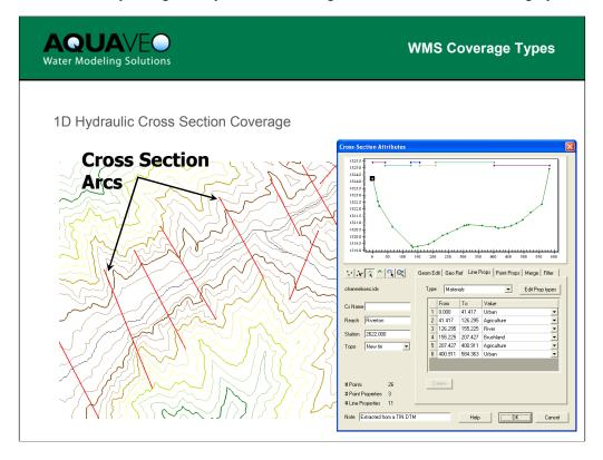
The 1D Hydraulic Cross Cection coverage is used to create cross sections in WMS. These cross sections can be used to determine the depth of water from the flow or the flow from the depth of water at any location in the watershed. These cross sections can also be used in any of the models that need cross sections to perform reach routing in WMS.
