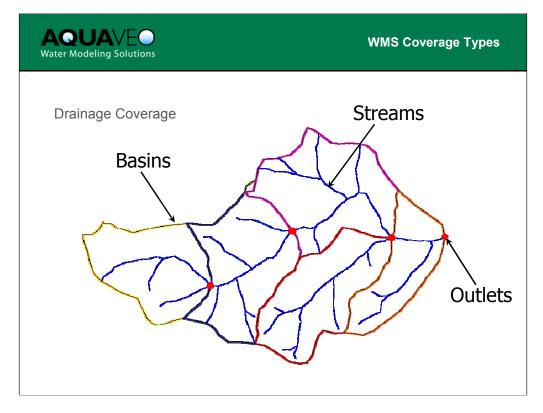
Drainage coverages are used for creating watershed models from feature objects and DEMs. They are slightly different than most coverages because they combine three separate layers in one: basins, streams, outlets. If you are performing watershed modeling, use a drainage coverage.
