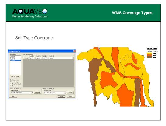
Soil type coverages are used to define soil type polygons for a watershed area. A soil type ID is assigned to each polygon. Each ID has a set of attributes that can be assigned to it. Soil type coverages can be used with land use coverages to compute composite Curve Numbers or Green-Ampt parameters.
