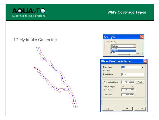
A 1D Hydraulic Centerline coverage is used to set up HEC-RAS and other hydraulic models. Centerline and bank arcs can be defined.
