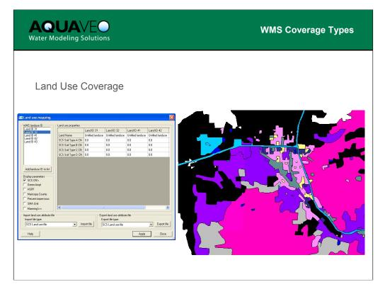
Land use coverages are used to define land use polygons for a watershed area. A land use ID is assigned to land use polygons. Then a table is set up that relates each ID to a set of land use attributes. The land use coverage can be used with a soil type coverage to compute composite Curve Numbers or Green-Ampt parameters.
