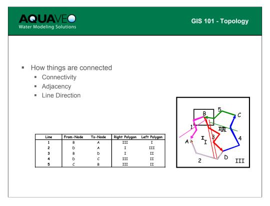
Topology is the way things are connected, or the spatial relationship between different features. For example, topology tells us how two lines are linked together and the direction we move along a line. It also tells us how polygons are formed so that we can identify lines within or adjacent polygons more simply. Topology should not be confused with topography, which defines surface features such as contours.
