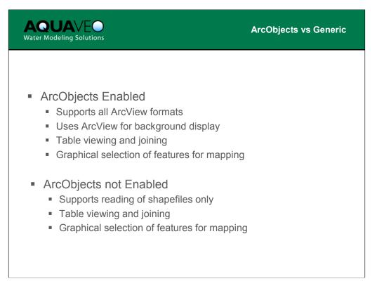
When ArcObjects is enabled, you can open any of the file types supported by ESRI's ArcView, including grids and images. If no license of ArcView is available then the GIS module can only be used to open and manipulate shapefiles.
