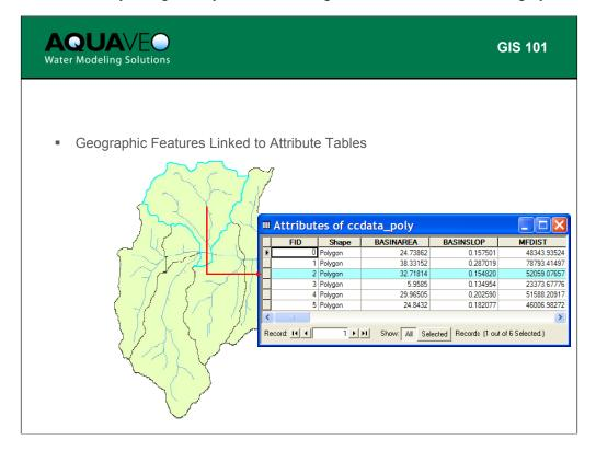
The basic genius of GIS is that geographic, or map features can be linked to a database. Essentially you can think of GIS as a database, but as part of the data structure the geographic shape and location are included. In simple terms you can think of GIS as CAD connected with a Database.
